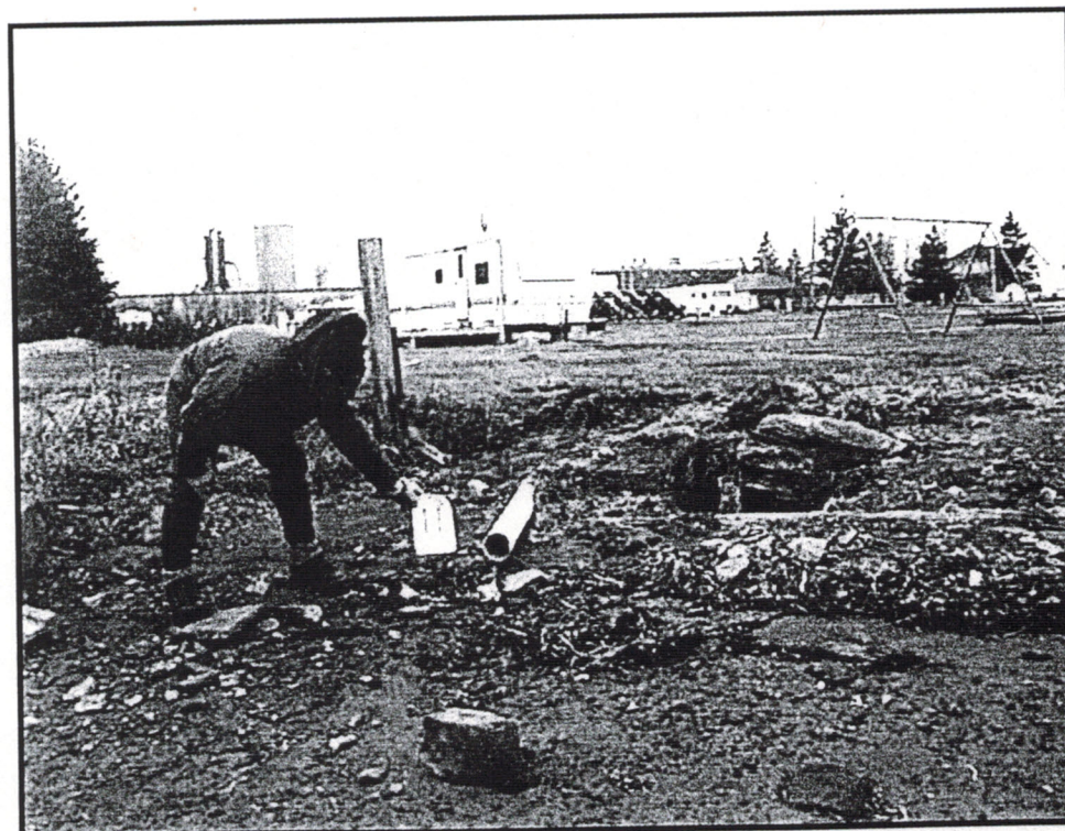
Figure 8. Plastic drainage pipe originating from trailer camp ground at site 11.
